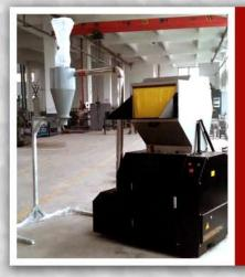
MACHTEK Plastic Granulators MG25 Series come with a blower and cyclone dust separator or with a practical bin.
