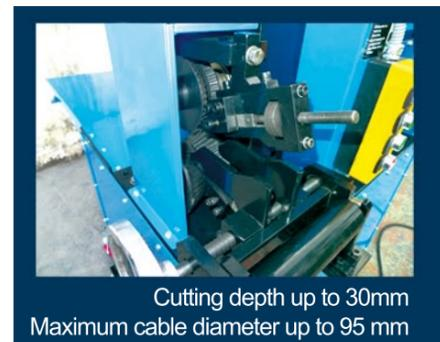
Cutting depth up to 30mm
